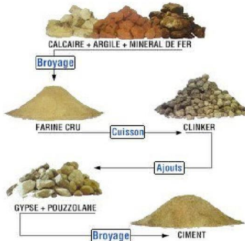
Figure II.13. Processus de fabrication de ciment.
