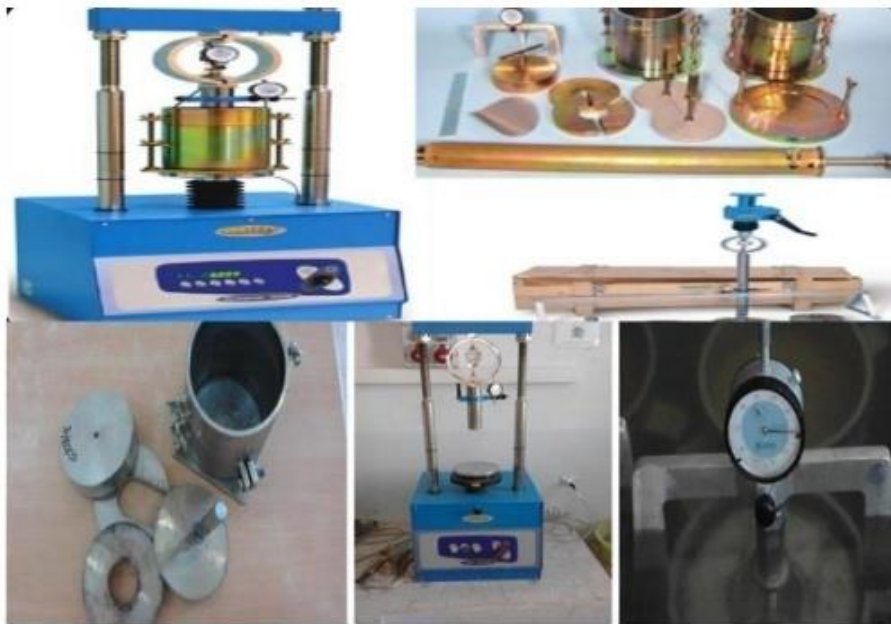
Figure III.25. L'essai CBR (California Bearing Ratio).
