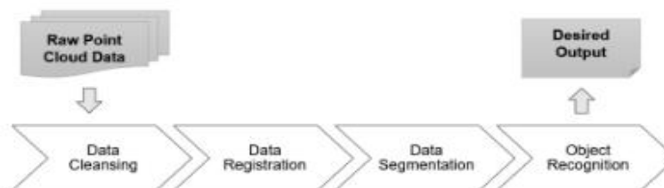
Figure 3.1. Typical processing procedures of point cloud data [30].
