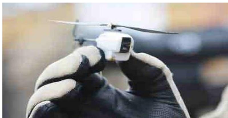
**Figure I.3 :** Le drone mono-rotor [1]
