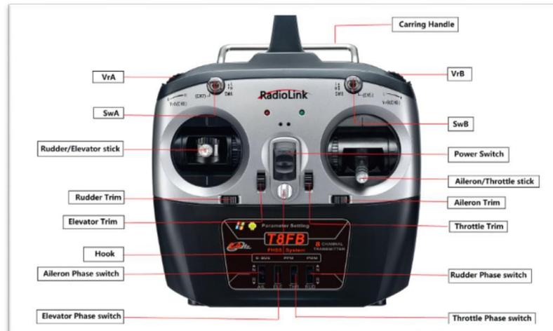
Figure III .8: Radiolink T8FB. [2]
