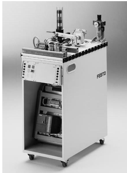
Figure IV.4: Distributing station with trolley, control console and PLC board
