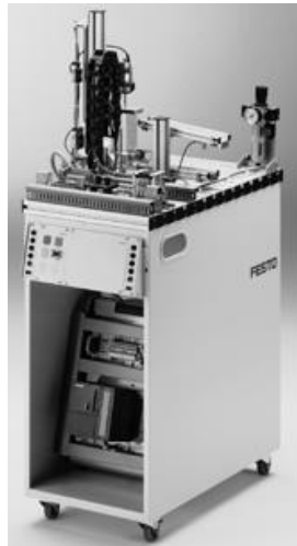
Figure IV.7: Testing station with trolley, control console and PLC board
