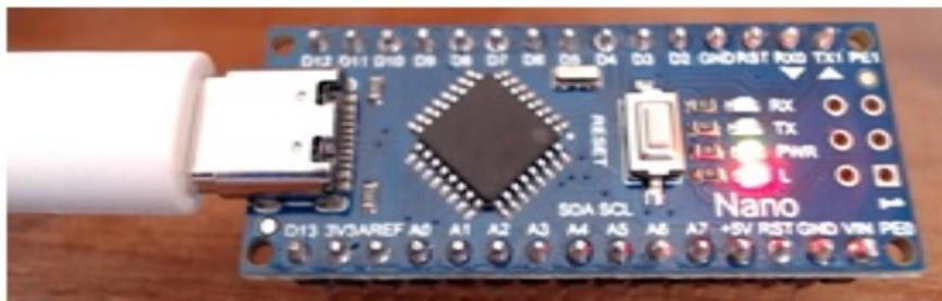
Figure.III.16: Programmeur Arduino Nano.
