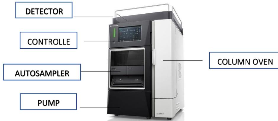
**Figure 10:** HPLC LC-2030C NT
