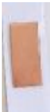
Figure II.4. Working electrode used in experimental set up (copper substrate).
