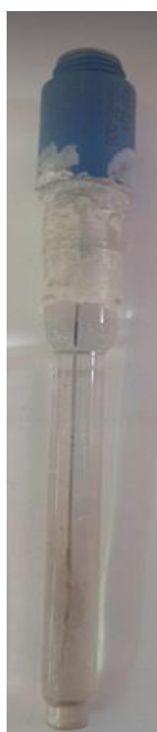
Figure II.5. Reference electrode Ag/AgCl electrode.
