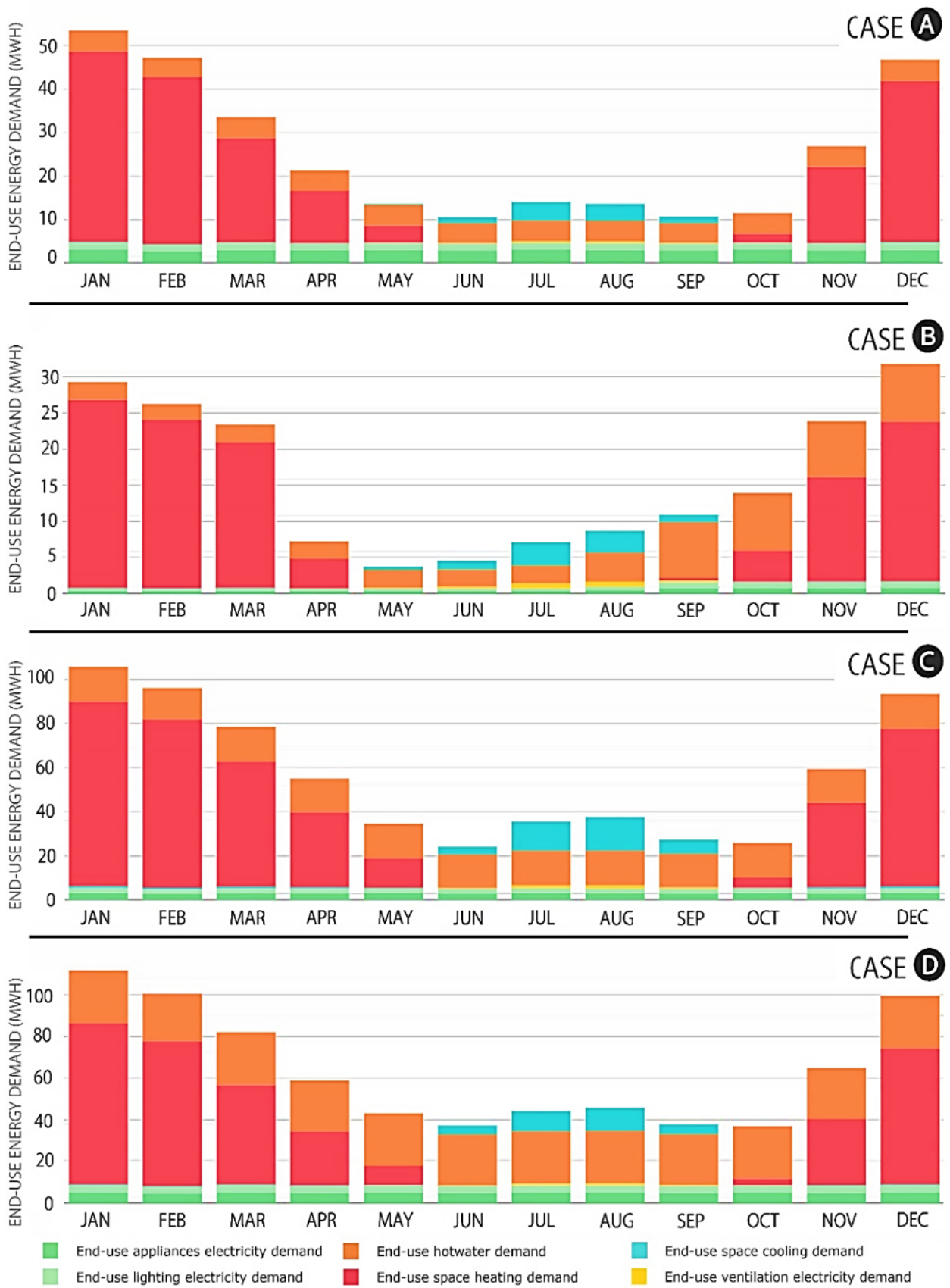
Figure VII. 13. Simulated monthly energy consumption bar charts, after calibration and validation.
