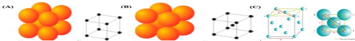
Figure II. 6. (A) La structure cubique simple (CS), (B) La structure cubique centrée (CC), (C) la structure cubique à faces centrées (CFC).
