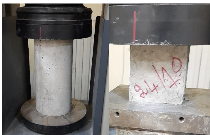
Figure III-1. Compression test specimens (cylindrical and cubic)
