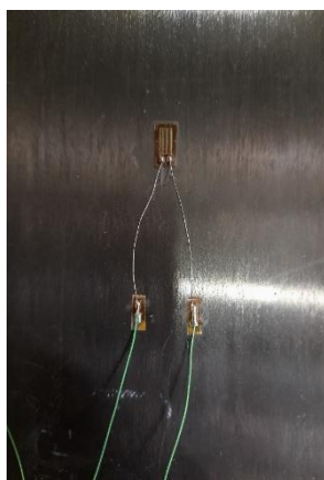
Figure III-16. strain gauge on CFRP laminate
