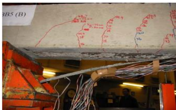
Figure II-17. FRP Plate end interfacial debonding [49].
