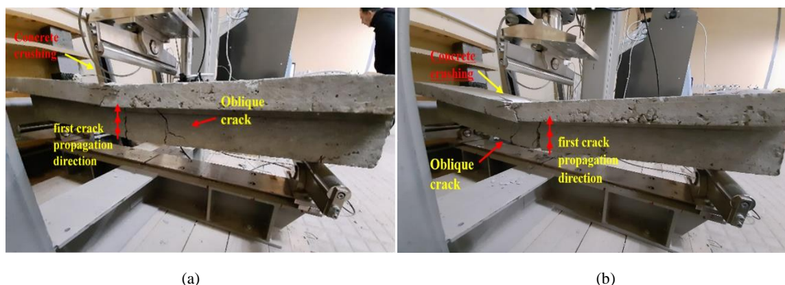
Figure IV-1. Crack Propagation and Failure Modes of Control Beams: (a) CB; (b) HCB
