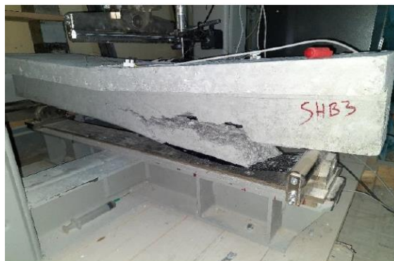
Figure II-16. Concrete cover separation of RC beam specimen strengthened by FRP (current study).
