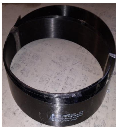
Figure III-4. CFRP laminate (Sika CarboDur S1012)
