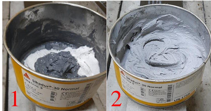
Figure III-5. Preparation of the resin
