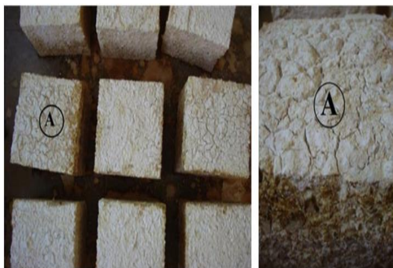
Figure I-8. Example of attack by sulfuric acid dosed at 5% for ordinary concrete for four months [18].
