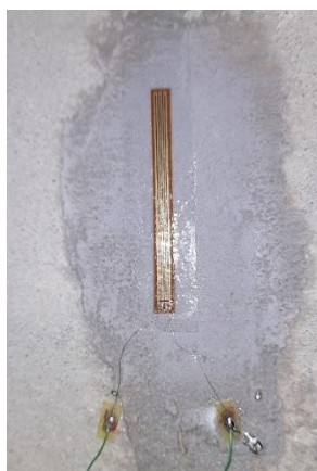
Figure III-15. strain gauge on concrete surface
