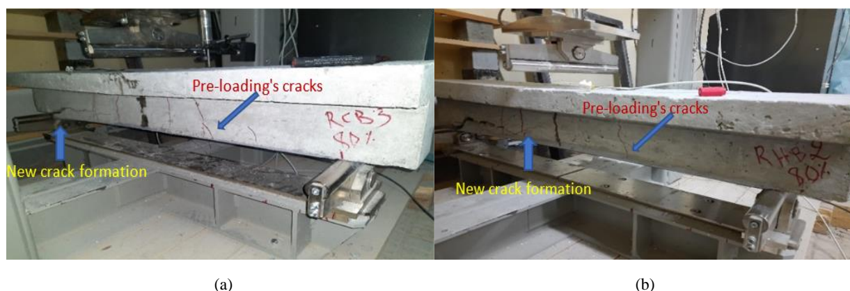
Figure IV-3. Crack Propagation and Mode of Failure of Retrofitted Girders: (a) RCB80; (b) RHB80
