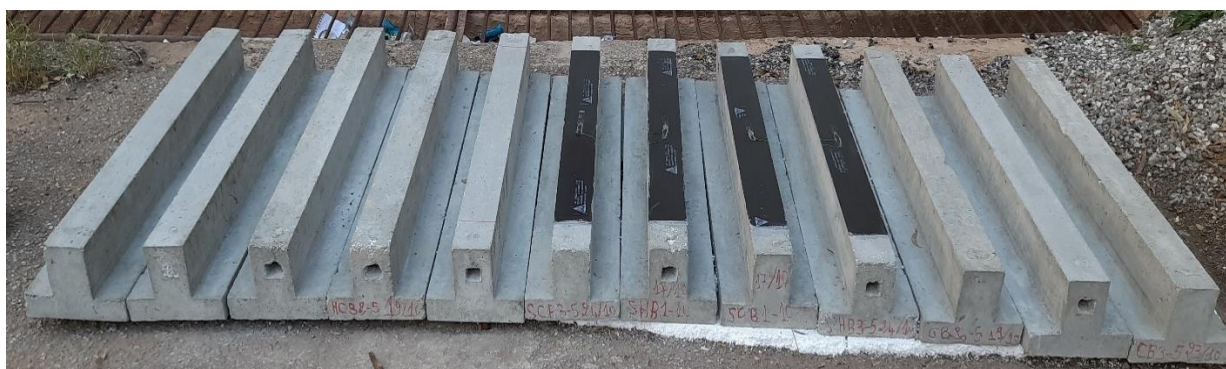
Figure III-7. experimental RC T-beams
