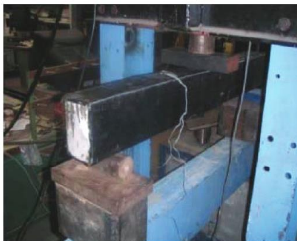
Figure II-10. Full wrapped RC beam by CFRP [41].
