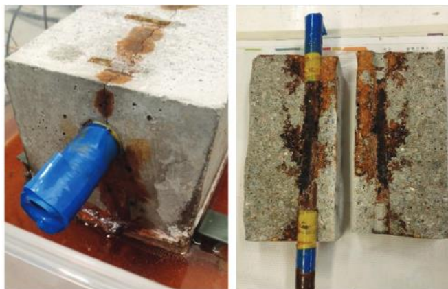
Figure I-13. Cracking Caused by Corrosion in Reinforced Concrete as a Result of Chloride Pollution and Ingress [28].
