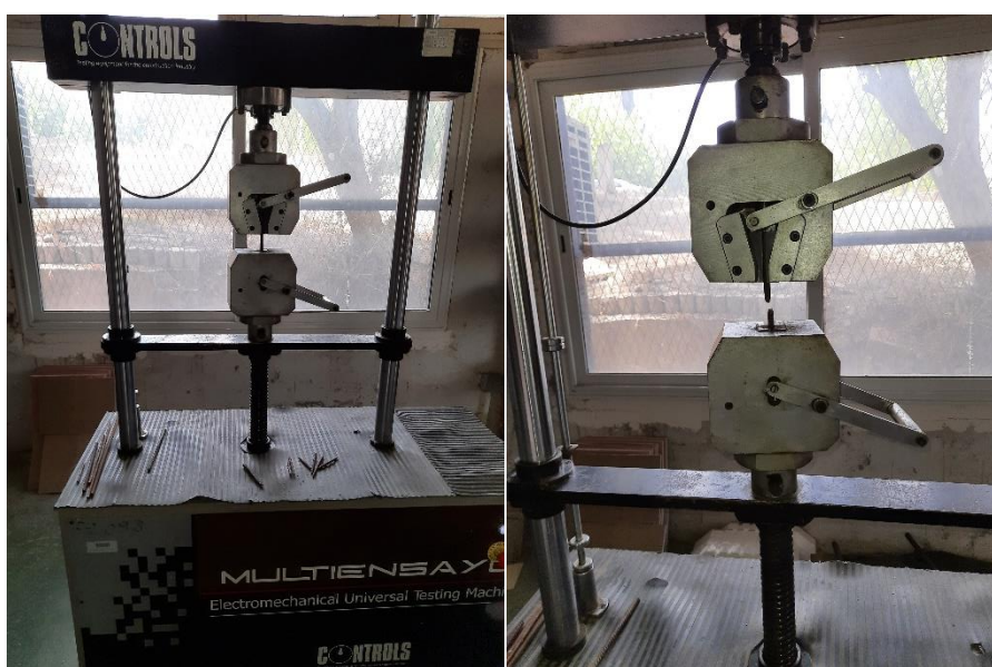
Figure III-3. tensile tests of reinforcements bars
