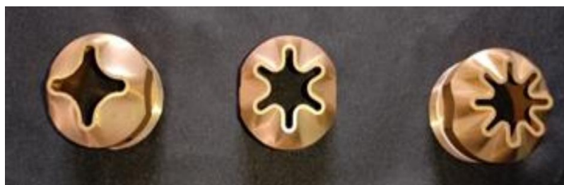
Figure 2.26: Corrugated lobed nozzles with 10mm, 15mm and 20mm lobe lengths (Roy et al., 2022)
