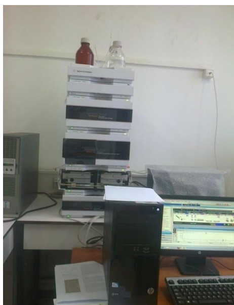
Figure III.4: (a) Appareil HPLC Agilent 1260 Infinity, (b) Composantes d'un appareil HPLC [3].
