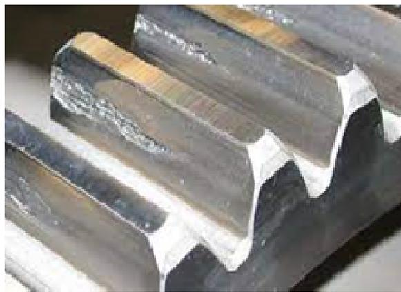
**Figure 1.8.** Worn gear.
