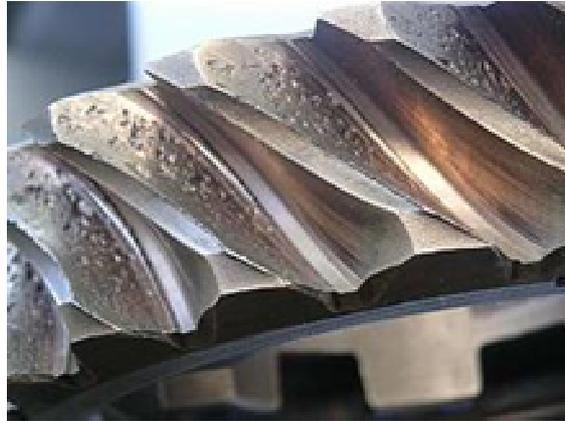
**Figure 1.10.** Deformation of teeth under overload.
