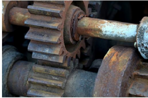
**Figure 1.11.** Corrosion.
