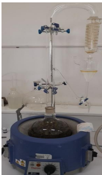
Figure 08: Clevenger apparatus used for essential oils extraction
