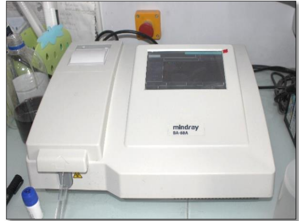
Figure 17: Reading of results using a Mindray spectrophotometer
