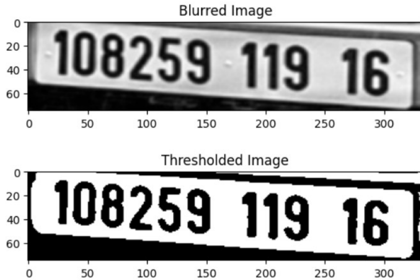
Figure 3.7: Example of Otsu's thresholding license plate .
