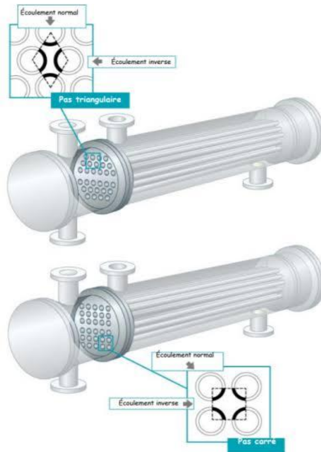
Figure II.3: Disposition des tubes [17] .
