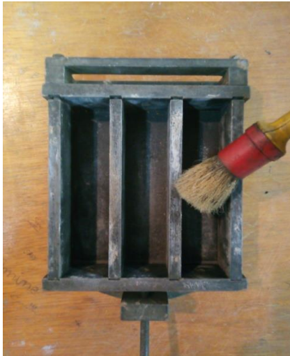
Figure III.21 : Lubrification des moules (4 x 4 x 16) cm 3 .
