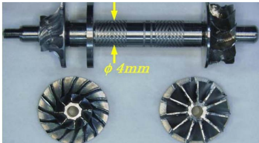
Fig. I.5 Grooved rotor of a micro turbomachine
