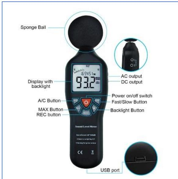
Figure 61: Sonomètre Triplett 3550 SoniChek Pro. Source: Amazon.com, 2022
