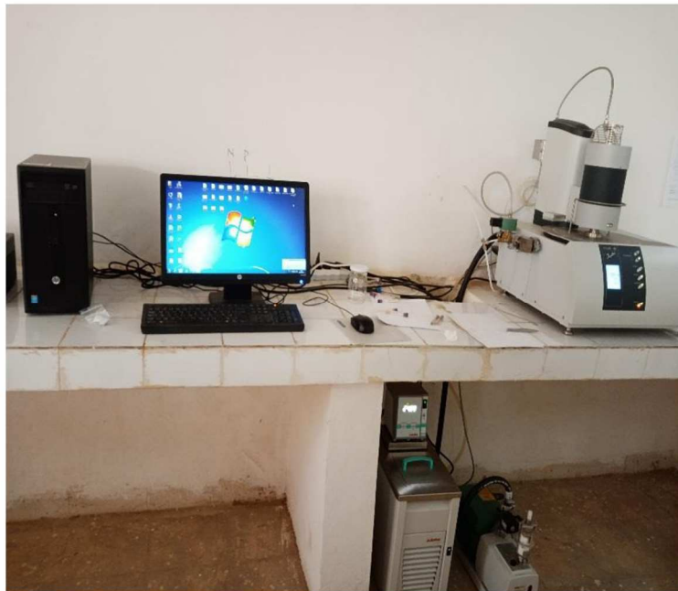
Figure III.10: Device (ATG/DSC) STA 449 (F3) -Jupiter
