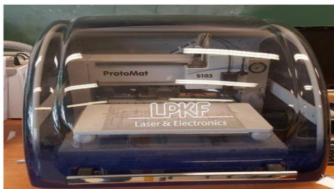
Figure (III.2) : La machine LPKFProtoMap S103.
