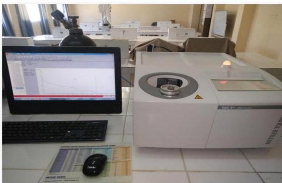
Figure III. 3: Machine de DSC de type METTLER TOLEDO DSC.
