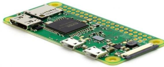
Figure 2.13: Raspberry pi zero w.
