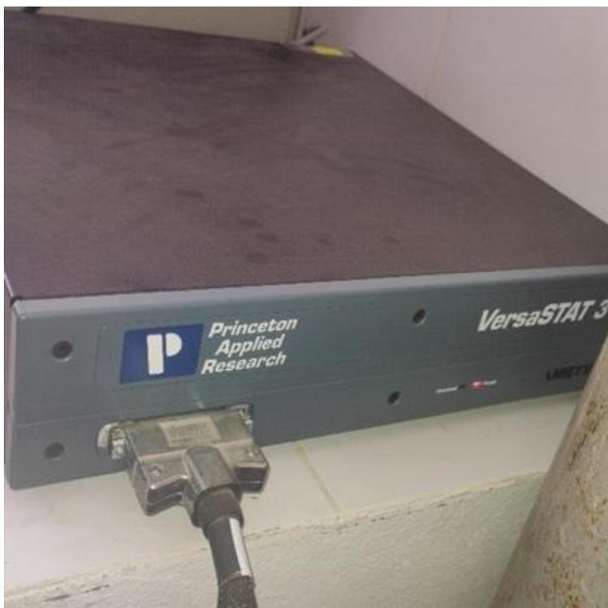
**Figure III.6 :** Potentiostat/Galvanostat
