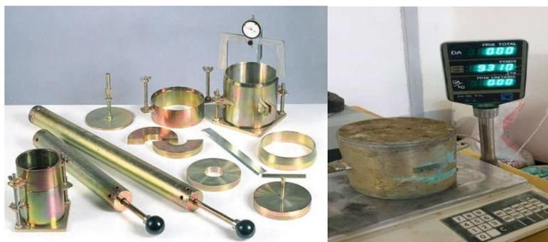
Fig. 39 Essai Proctor normal
