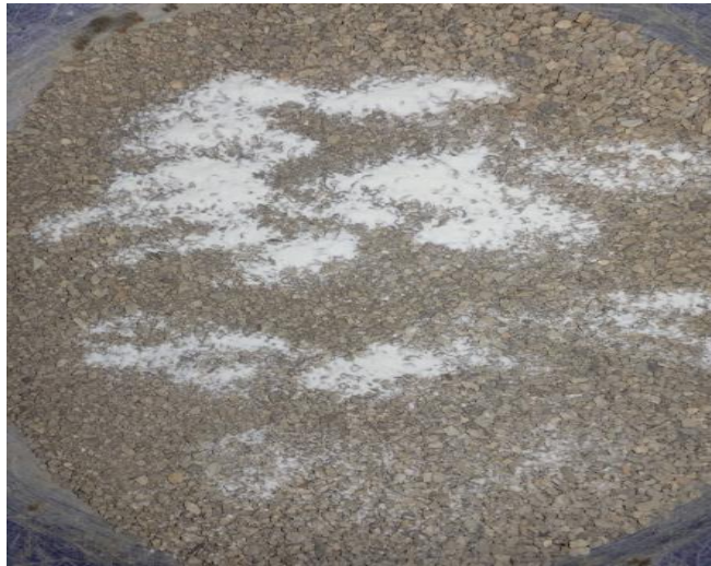
Figure 4.25 Mélange sol-bioliant à sec
