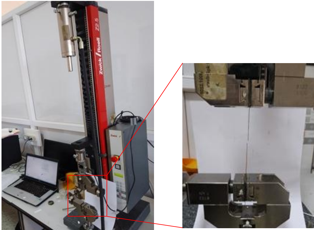
Figure II.12: Machine de traction universelle type Zwick / Roell Z2.5
