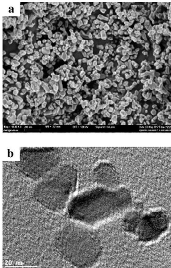
**Figure 5- 7:**(a) Image SEM de nanoparticules de TiO<sub>2</sub>, (b) image TEM de nanoparticules de TiO<sub>2</sub>. [55]
