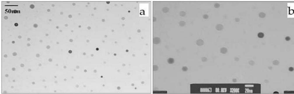
**Figure 5- 6:**(a) Image FE-MEB de nanoparticules de TiO<sub>2</sub>; (b) Image MET du nanofluide TiO<sub>2</sub>[54].
