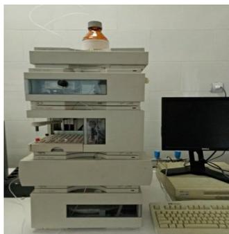
**Figure IV.16 :** chromatographe phase liquide.
