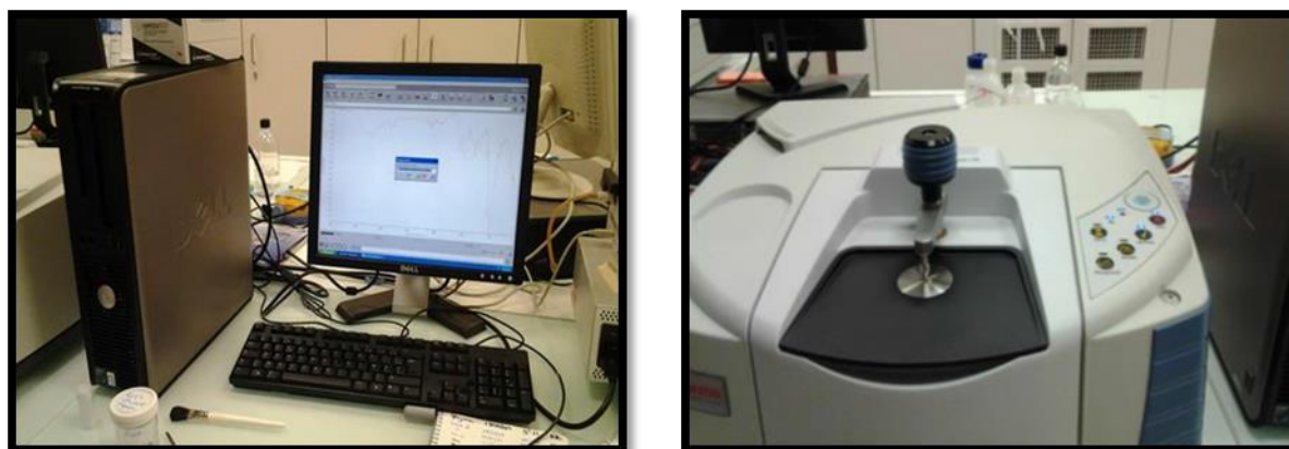
Figure IV. 9: Spectromètre IR-TF Nicolet iS10 (ThermoFischer Scientific).
