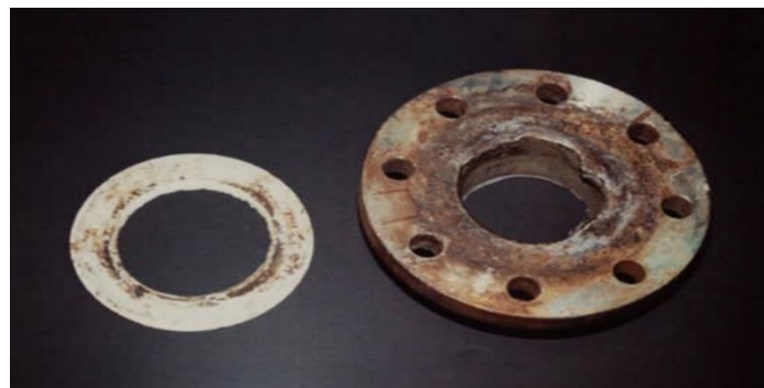
Figure I.4. La corrosion caverneuse [9]
