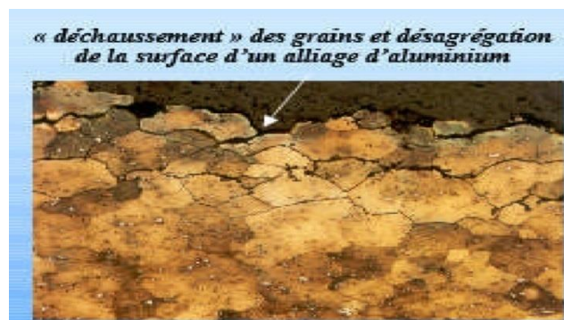
Figure I.6. La corrosion inter-granulaire [9]
