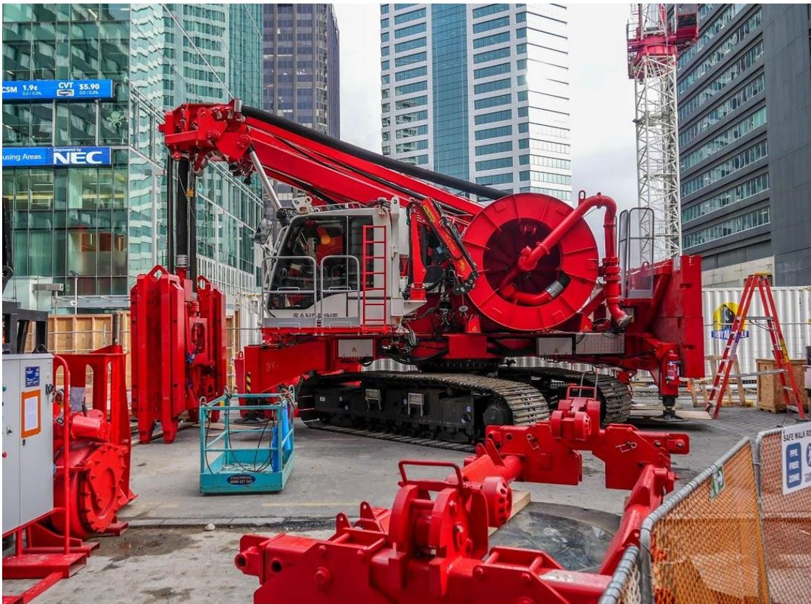
Figure I.20 : hydrofraise
