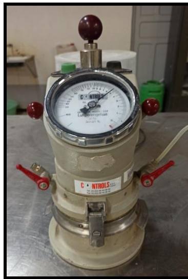
Figure II.13 : Essai teneur en air occlus.
