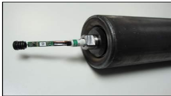
Figure III.7 Le rouleau du support intelligent.
