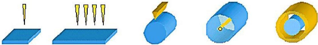
*Pointe/Plan Multipointe/Plan Couteau/Cylindre Fil/Cylindre Cylindre/Cylindre*
