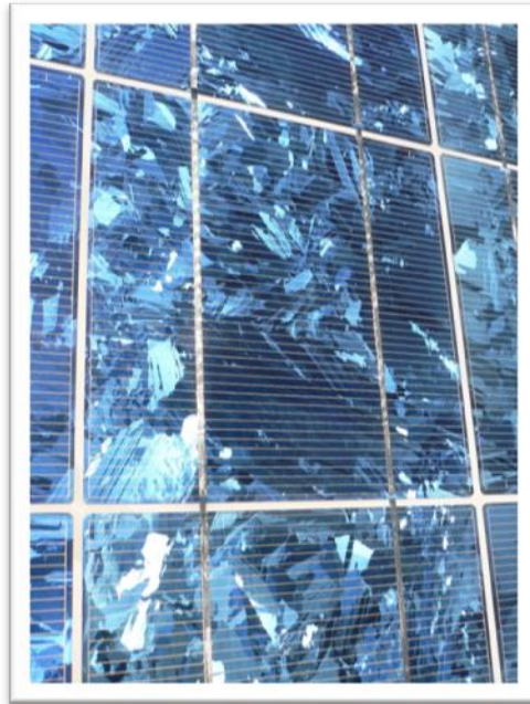
FIGURE I.4: Cellule photovoltaïque poly-cristalline.
