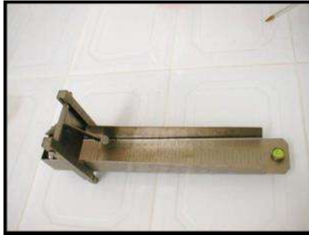
Figure 10: Consistomètre de Bostwick (Boumendjel et al., 2012).
