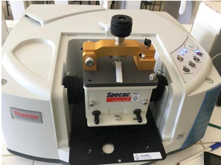
Figure III.8: Appareille FTIR ATR SPECAC IS10.
