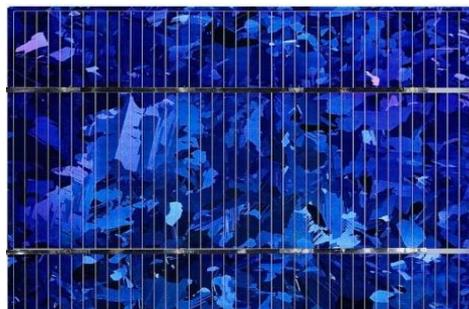
Figure I-7: cellule PV poly-cristallin.
