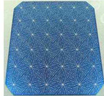
**Figure I.6** Cellule MWT [8]
