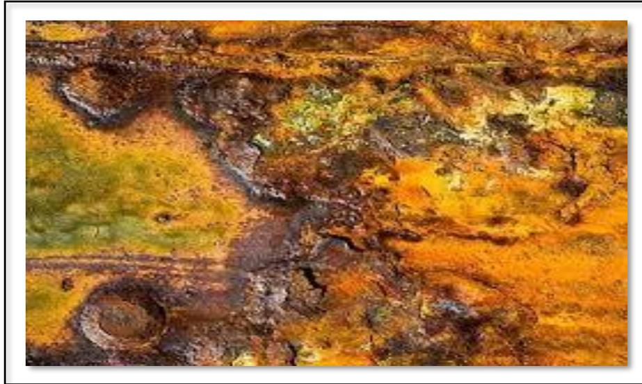
**Figure 2.14:** Corrosion uniforme [AFGC 03].
